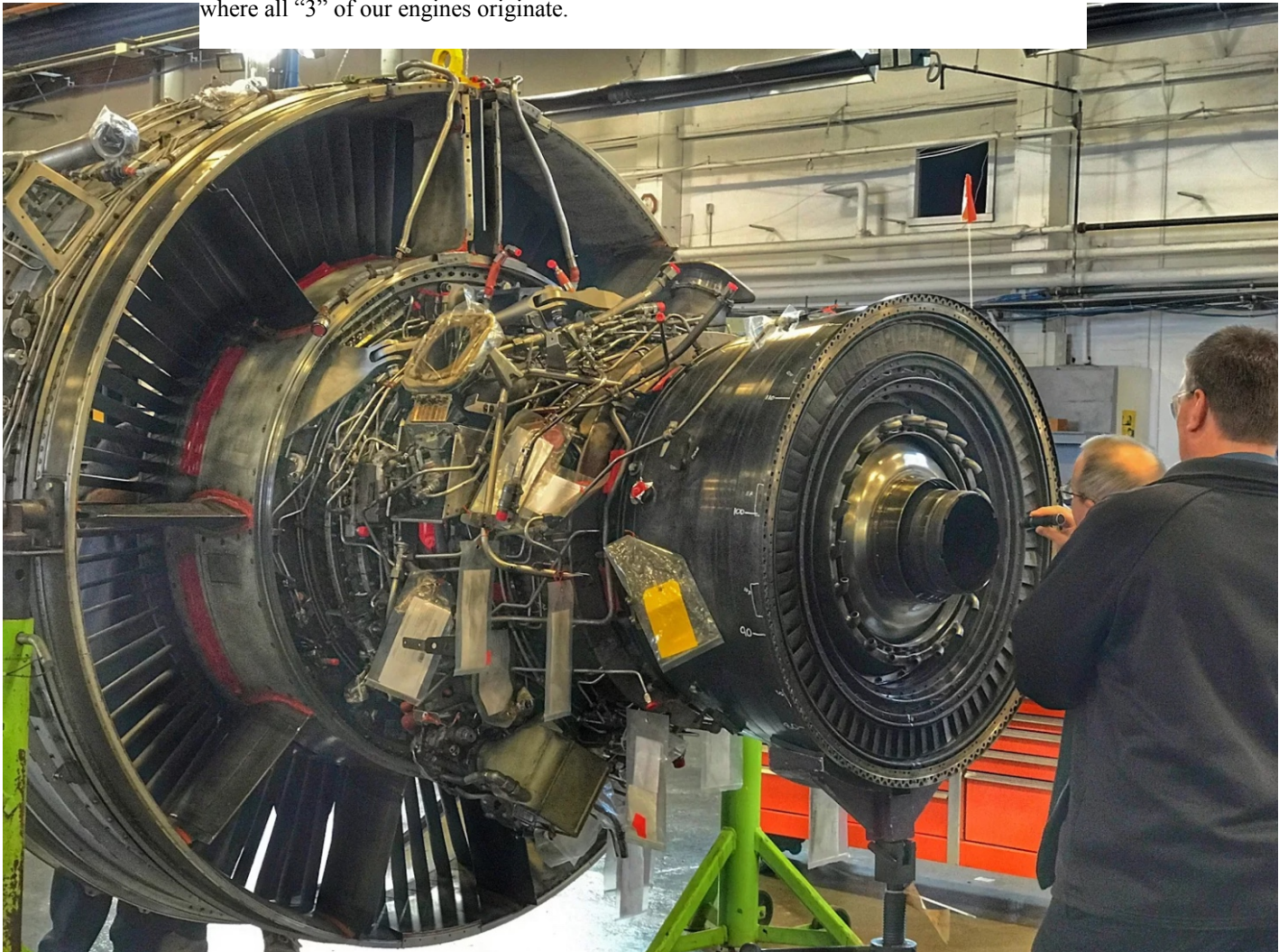
"Doing a final area inspection of the aft end of the Diffuser case/Combustion module, before installing the HPT over top of it . Can't have any foreign crap floating around in there. Pratt JT9D-7R4D assembly." Photo by Fred Robel. Source : Google+ more (emphasis added) This is the exact model of engine used on Flight 175.
